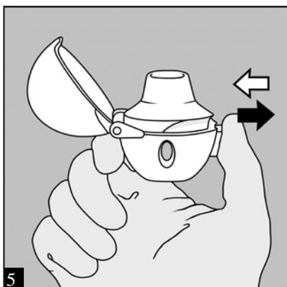
**PRESS: Hold the HandiHaler with the mouthpiece upwards and press the piercing button completely in only once until it is flush against the base, and release.**
